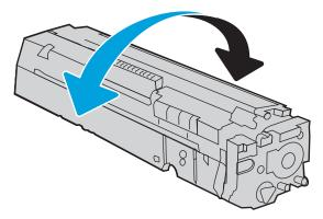
7. Do not touch the imaging drum on the bottom of the toner cartridge. Fingerprints on the imaging drum can cause print-quality problems. Also, do not expose the cartridge to light unnecessarily.
