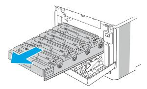
3. Grasp the handle on the toner cartridge, and then pull the toner cartridge straight up to remove it.
