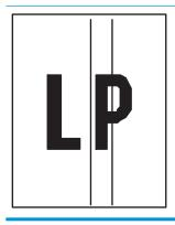
Dark vertical lines which occur down the length of the page. The defect might occur anywhere on the page, in areas of fill or in sections with no printed content. On color models, these lines or streaks will also be visible on the ITB cleaning page.
