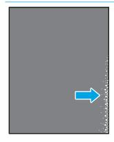
Toner rubs off along either edge of the page. This defect is more common at the edges of high-coverage jobs, and on light media types, but can occur anywhere on the page.
