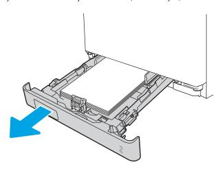
3. At the left side of the Tray 2 cavity, press the tab to lower the tray plate, and then remove any paper. Remove the jammed sheet by gently pulling it straight out.
